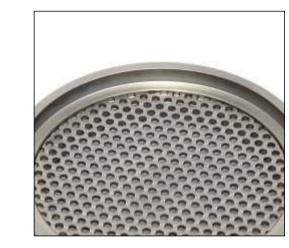
Sample preparation needs a spoonful of diatomite (Kieselgur) only. Pour in juice sample, close the lid and start air compression. Approximately 30 seconds later, depending on product, the clear filtrate is ready for use in a NIR polarimeter. After decompression simply remove filter cake and start next filtration.
