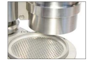
Pressure filtration with ZORN's ZPF 2.0 works much faster than conventional methods. Preparation of a juice sample takes less than one minute. Waiving of chemical clarifying agents allows for the pol and Brix analysis to be carried out with the same sample. Apart from the increase in efficiency use of the ZPF 2.0 further safes cost as the filter-cel grade diatomite (Kieselgur) used for filtration can be disposed of as standard, non-hazardous waste.
